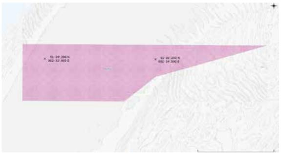
Shipping is made aware of the presence of telecommunication and export cables just above the northern limit of the anchor area Oostdyck. When anchoring, sufficient account must be taken to keep the anchor within the limits of the Oostdyck anchor area.
