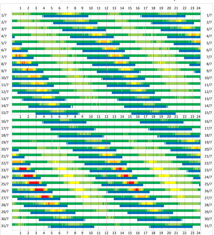
Predicted current speed at the Nieuwpoort flood barrier based on astronomic tide data during the construction phase
